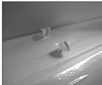
Figure 8 – Affix the air-cleaner wing nut on the bottom spine
