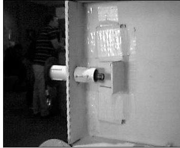
Figure 5 – Hole for the flashlight insertion tube goes on the left box spine
