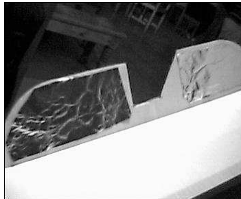
Figure 6 – Notch the flap in the box lid to prevent interference with the flashlight insertion tube
