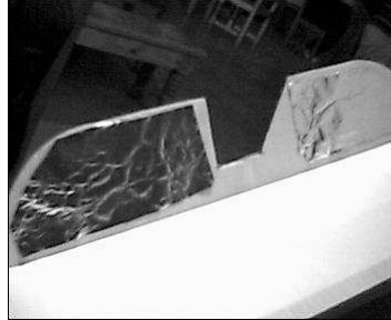
Figure 11 – Covering the inside left-hand flaps with reflective material
